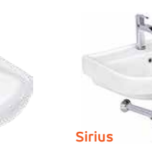
Sirius WM-22-X / WM-22-G* Wall mounted basin 565x420x200 Rack Bolt distance: 230 mm / 215 mm Tap Hole dia: 35 mm / 35 mm ₹1850 / ₹1700 Compatible with full pedestal FP-22-X ₹2000
